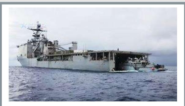
Here's the USS Comstock LSD-50 with a Mark VI patrol Boat entering her well deck. The radar mast folds down to clear the flight deck. The "New" Carter Hall is in the same class. One major improvement is the Flight Deck is the full width of the ship Making it much larger.
